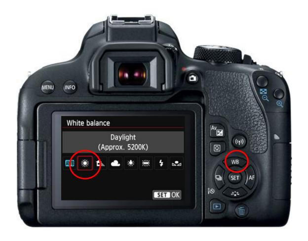
PRESS THE WHITE BALANCE SELECTION BUTTON AND USE THE MAIN DIAL TO ADJUST TO DAYLIGHT (5200K)
