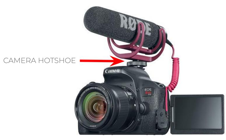
ATTACH THE RODE MIC TO THE CAMERA HOTSHOE AND PLUG THE MIC CABLE INTO THE MIC INPUT AS SHOWN
